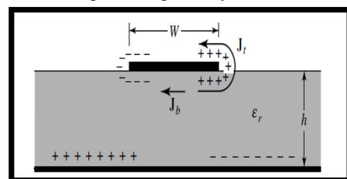
Fig. 1. Charge distribution and current density creation on microstrip patch [7].
