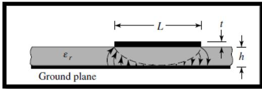
Fig. 2. Electric Field Lines on microstrip patch [7].
