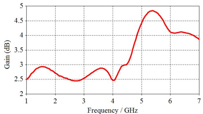
Fig.8. Gain vs Frequency of the proposed diamond Sierpinski MIMO fractal antenna
