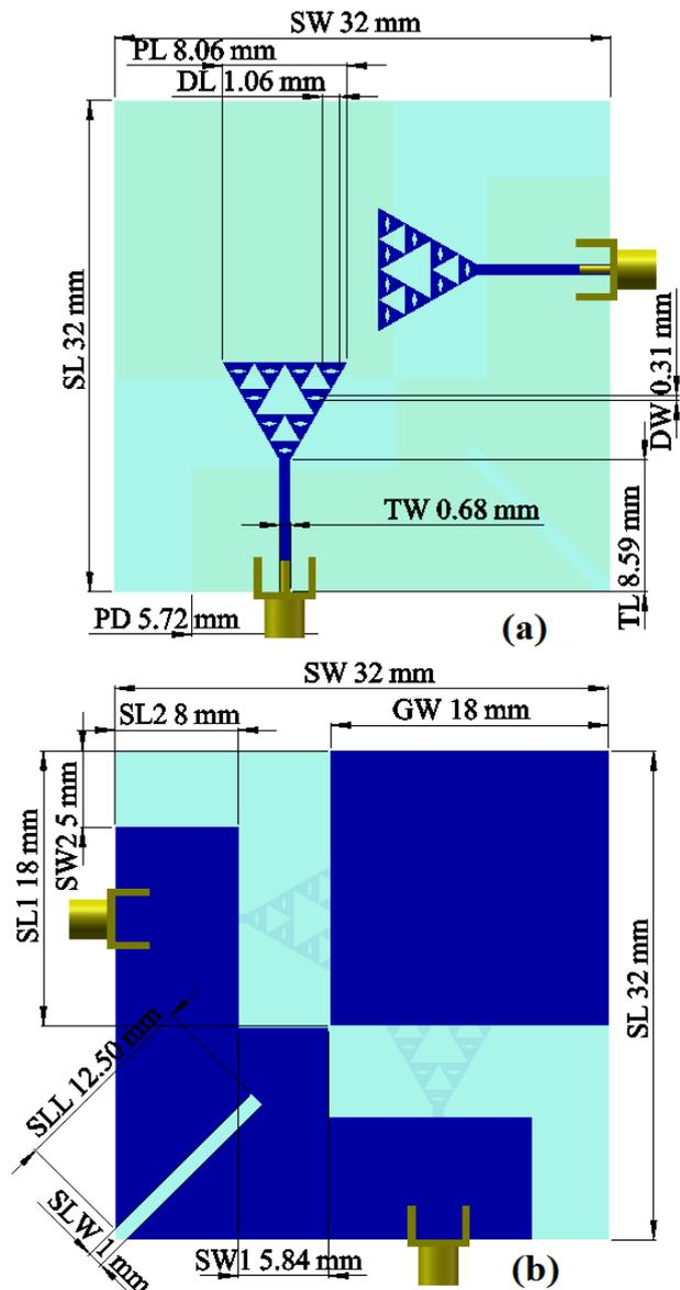
Fig.2. Dimensions Diagram of the proposed MIMO Diamond Sierpinski Fractal Antenna, (a) Top Layer, (b) Bottom Layer.
