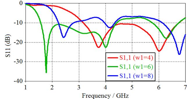
Fig.5. Frequency response of proposed diamond Sierpinski MIMO fractal antenna with respect to the slot width l
