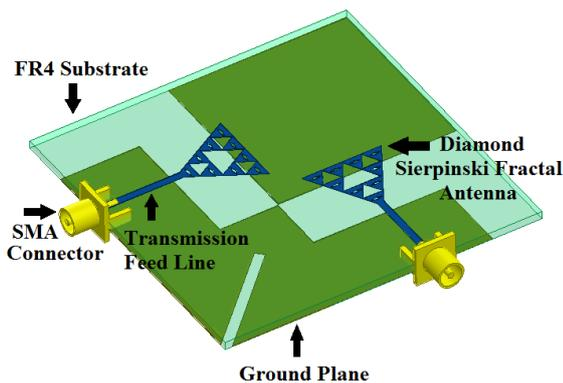
Fig. 1. Proposed MIMO Dual Element Diamond Sierpinski Fractal Antenna labeled diagram
