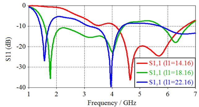
Fig.4. Frequency response of the proposed diamond Sierpinski MIMO fractal antenna with respect to the slot length l
