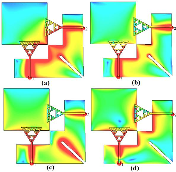
Fig.9. Surface currents of proposed diamond Sierpinski MIMO fractal antenna for frequencies, (a) 1.8 GHz, (b) 2.4 GHz, (c) 3.8 GHz, (d) 5.8 GHz.
