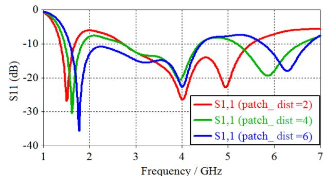
Fig.6. Frequency response of proposed diamond Sierpinski MIMO fractal antenna with respect to the patch distance from the ground plane slot
