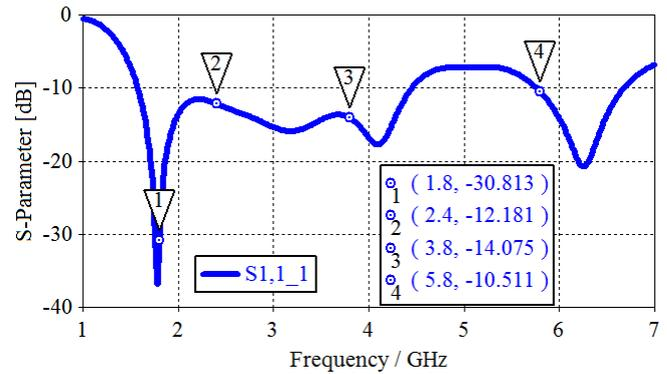
Fig.3. S11 Frequency Response of proposed Diamond Sierpinski MIMO fractal Antenna
