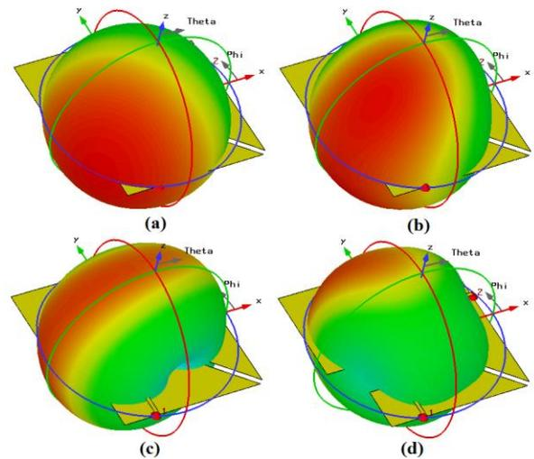
Fig.7. 3D Radiation Patterns of the proposed diamond Sierpinski MIMO Fractal Antenna for the frequencies, (a) 1.8 GHz, (b) 2.4 GHz, (c) 3.8 GHz, and (d) 5.8 GHz
