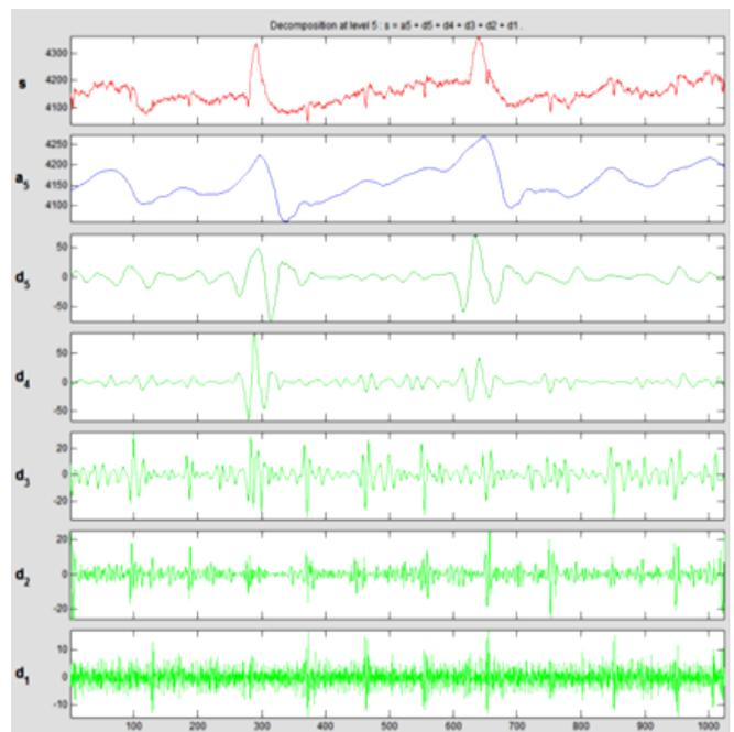
Fig.3: Show the 5 level decomposition of eye blink signal from d1 to d5 and the approximated signal a5.
