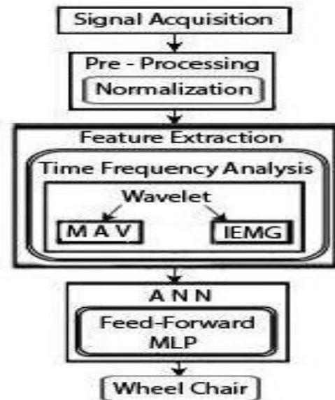
Fig.1: Proposed model for facial controlled wheelchair
