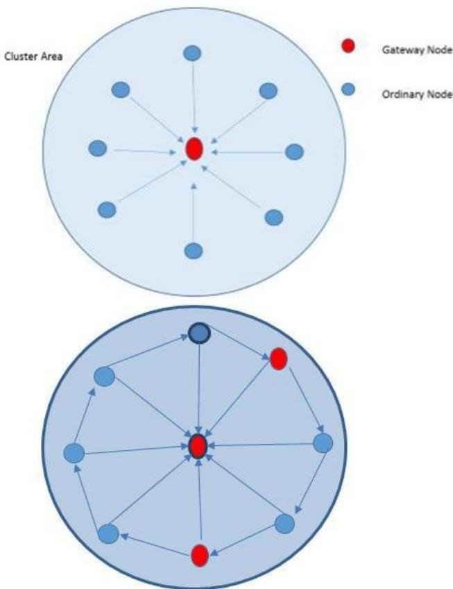
Fig. 1: (a)Centralized Realization Technique Architecture (b)Distributed Realization Technique Architecture
