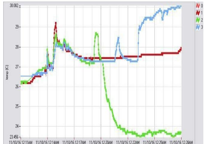
Fig. 7: Variation in Temperature to Time from MDA 100 system
