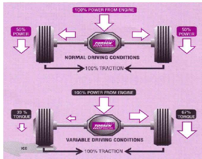
Fig. 1: distribution of torque according to slip of each wheel.
