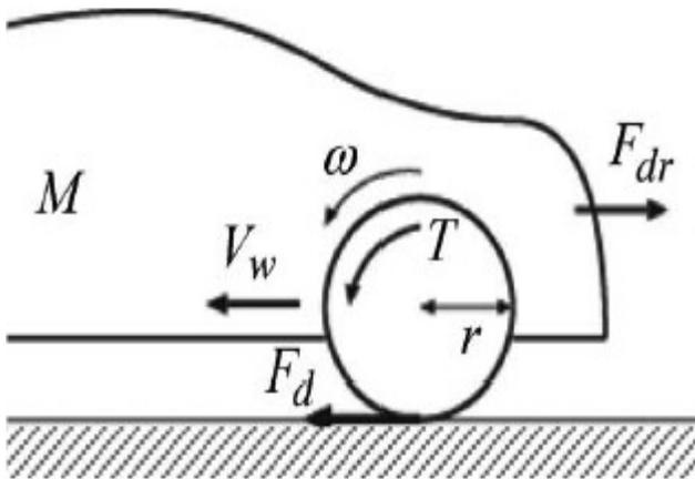
Fig. 2: Half vehicle longitudinal Model
