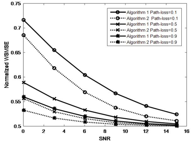
Fig. 4: Effect of power path-loss on Two Algorithms
