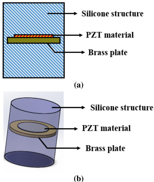
Fig. 1. Energy harvesting piezoelectric vibration isolator (a) Cross-sectional view (b) 3D model
