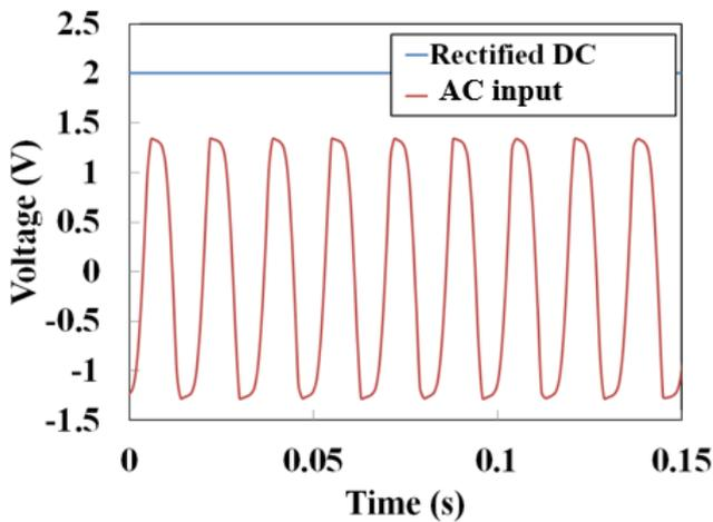
Fig. 8. AC Input from the energy harvesting piezoelectric vibration isolator and rectified DC voltage
