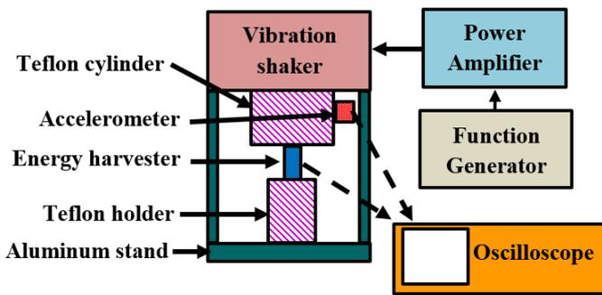
Fig. 3. Schematic of testing setup developed for the testing of energy harvesting vibration isolator
