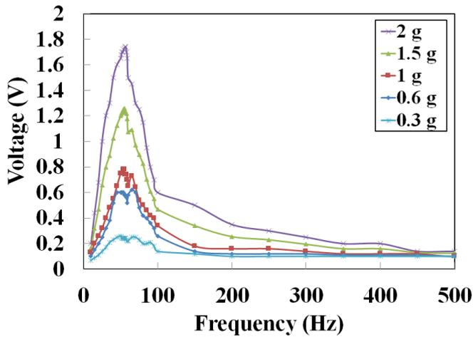
Fig. 4. Frequency versus voltage response of energy harvesting piezoelectric vibration isolator
