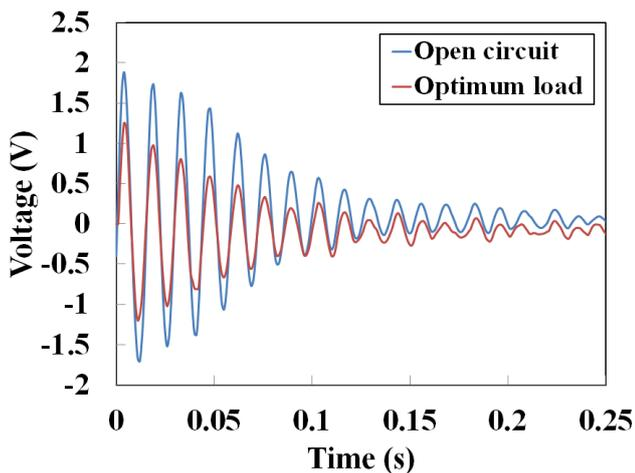
Fig. 9. Device free vibration response with open circuit and optimum load
