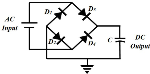
Fig. 7. Schematic of Wheat Stone Bridge Rectifier
