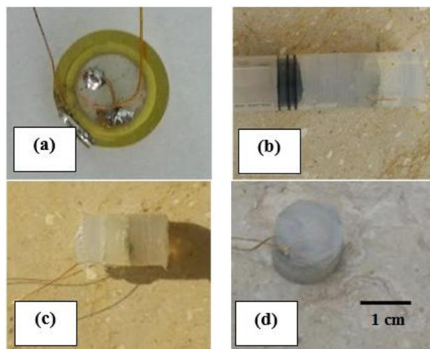
Fig. 2. Energy harvesting piezoelectric vibration isolator fabrication steps (a) Unimorph piezoelectric plate (b) Piezoelectric material deposited plate embedded in uncured silicone (c) Cured silicone structure (d) Finished energy harvester
