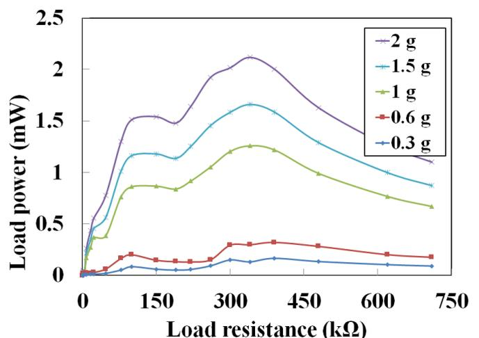
Fig. 6. Load power versus load resistance at different acceleration levels
