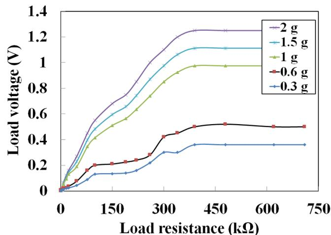
Fig. 5. Load voltage versus load resistance at different acceleration levels
