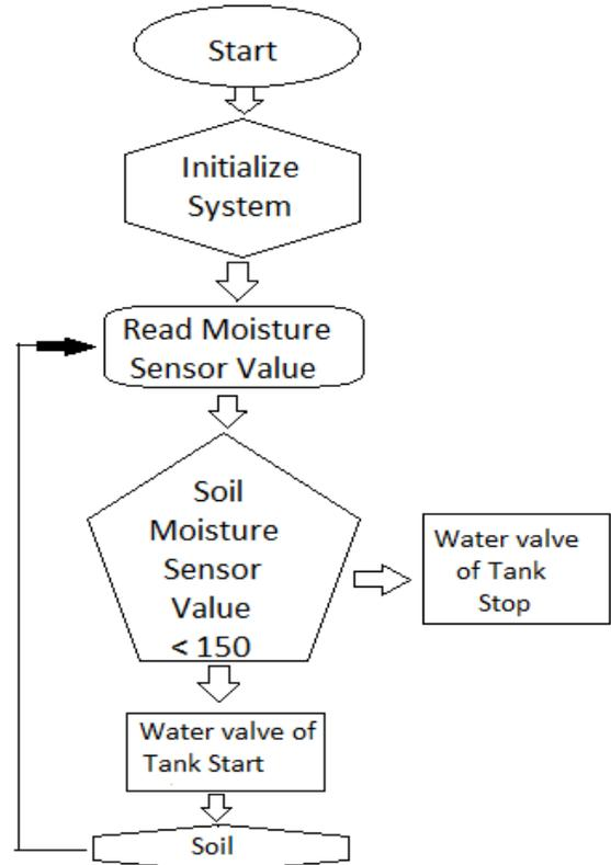
Fig. 9. Flow Chart of regulating water
