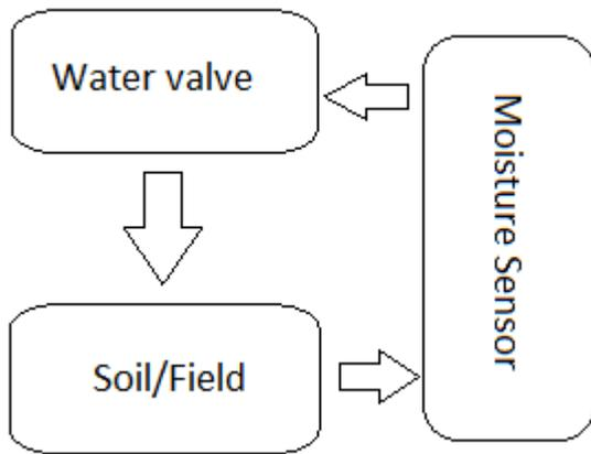
Fig. 8. Electronic controlling of water valve
