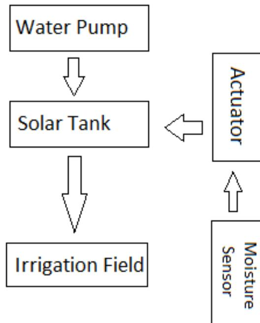
Fig. 7. Mechanism for Automatic irrigation module
