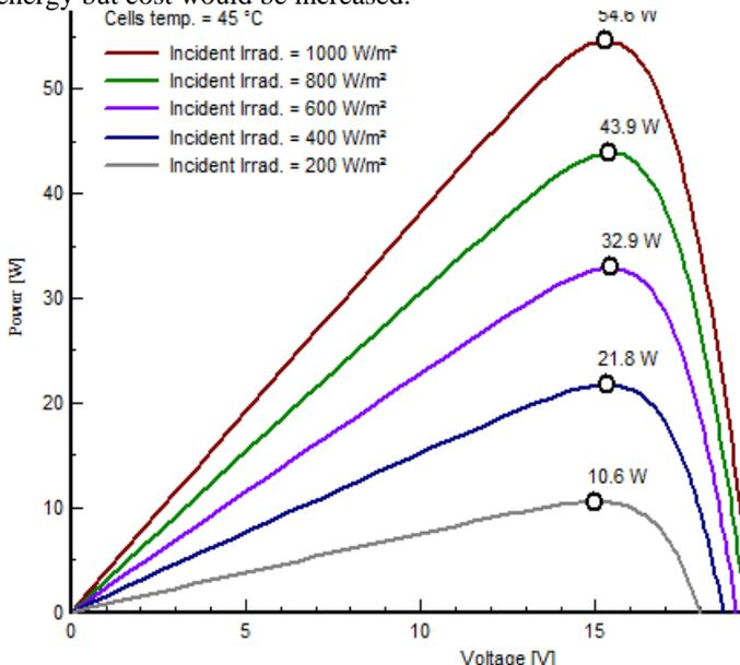
Fig. 14. Irradiance vs panel's output
