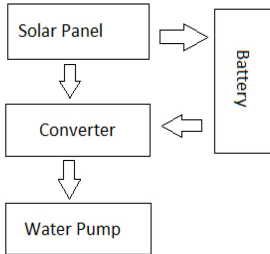
Fig. 6. Solar Pumping Mechanism
