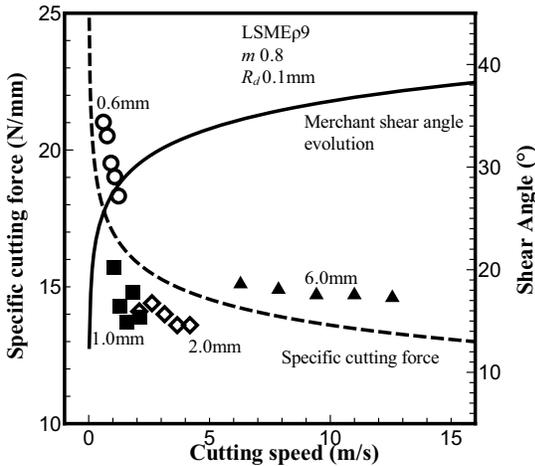
Figure 13: Effect of cutting speed on specific cutting force and Merchant shear angle evolution
