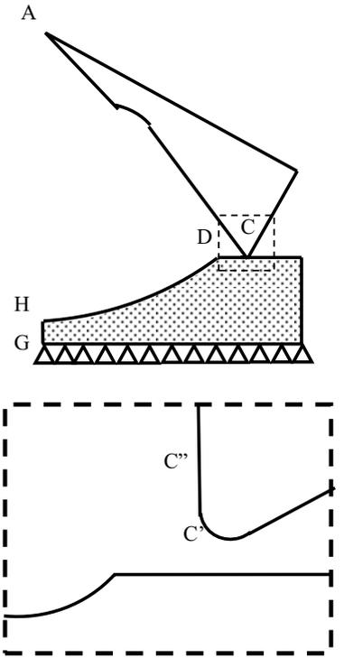
Figure 4: Thermal boundaries on tool and workpiece
