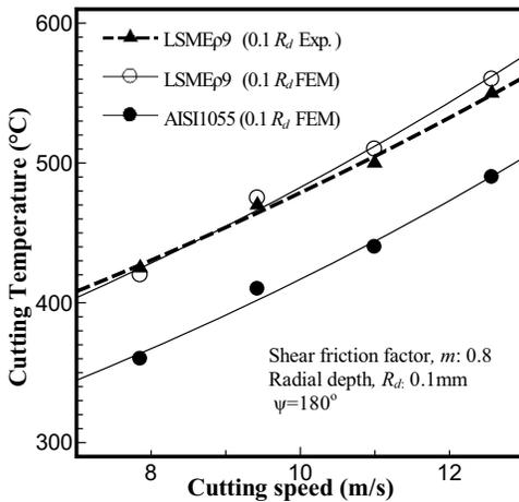
Figure 10: Effect of cutting speed on cutting temperature
