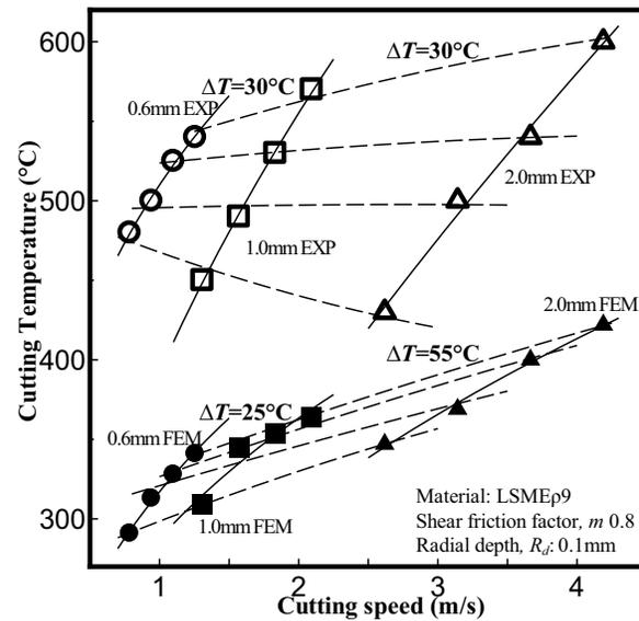
Figure 12: Comparison between estimated cutting temperatures with the experiment
