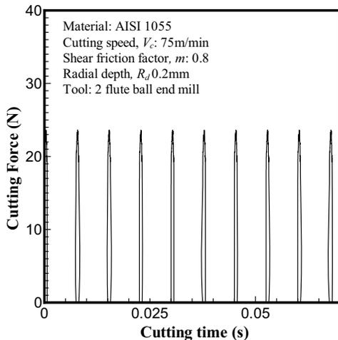
Figure 6: Cutting force profile
