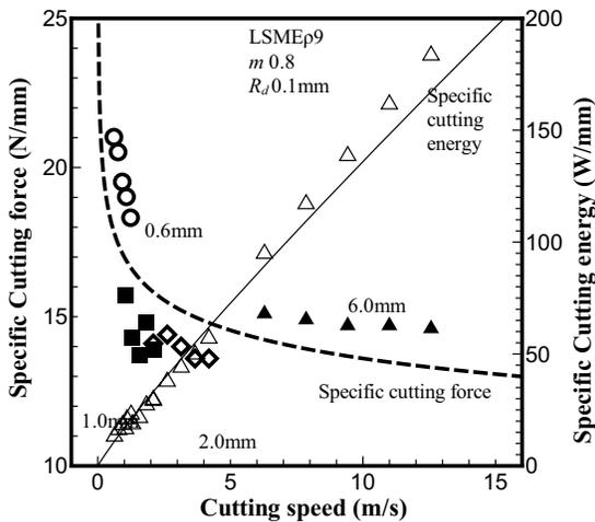
Figure 14: Effect of cutting speed on cutting force and cutting energy
