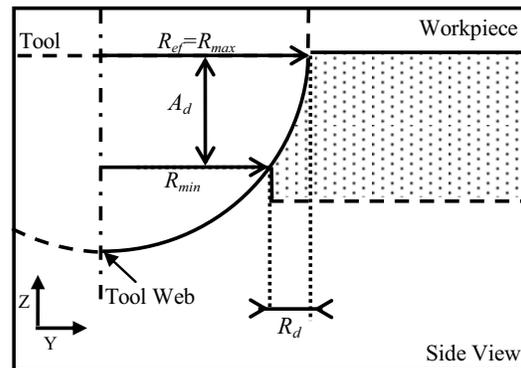
Figure 2: Peripheral milling on side view
