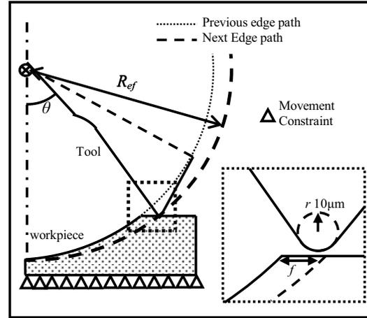
Figure 1: Simplified tool and workpiece FEM model
