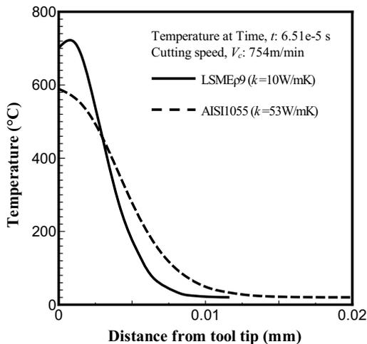
Figure 11: Temperature distribution comparison for different thermal conductivity
