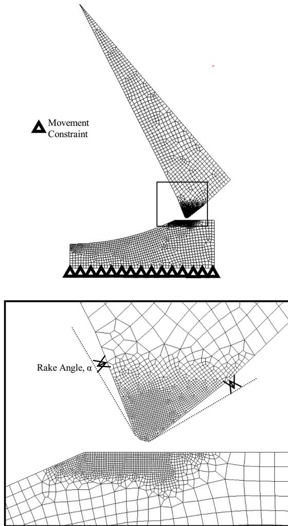
Figure 3: Model meshing and density
