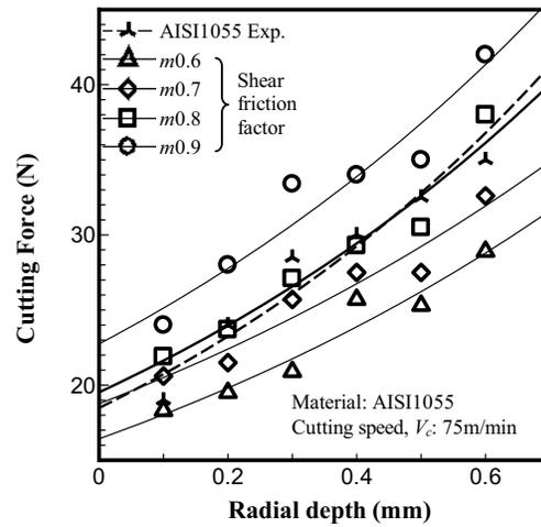
Figure 7: Effect of frictions model and radial depth on cutting force
