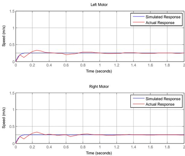
Fig. 6(a) Step Response for Speed = 0.25 m/s
