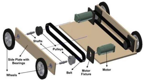
Fig.2. Detonated view of the platform CAD model of the prototype design
