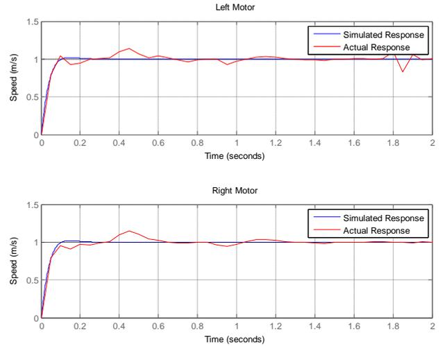
Figure 6(c) Step Response for Speed = 1.0 m/s
