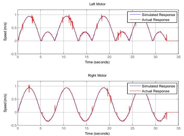
Fig. 7(a) Trajectory Tracking Response along Square Path
