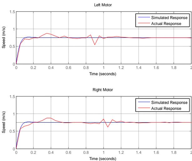
Fig. 6(c) Step Response for Speed = 0.75 m/s
