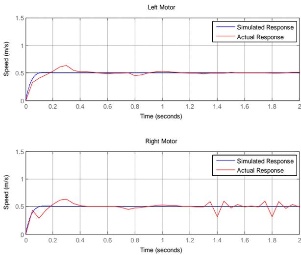
Fig. 6(b) Step Response for Speed = 0.5 m/s
