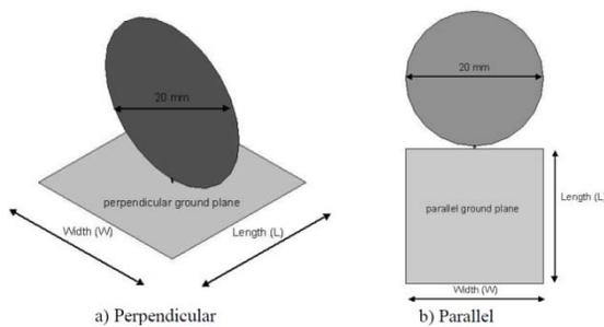
Figure 1: Printed Circuit Board monopole stack parameters
