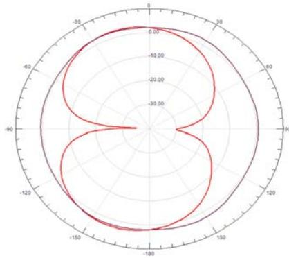
Figure 9. Radiation pattern of proposed antenna
