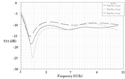
Figure 7. Showing the results of simulated return loss of rectangular antenna for different values of Wg
