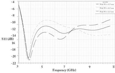
Figure 4: Showing the results of simulated return loss of rectangular antenna for different values of W1
