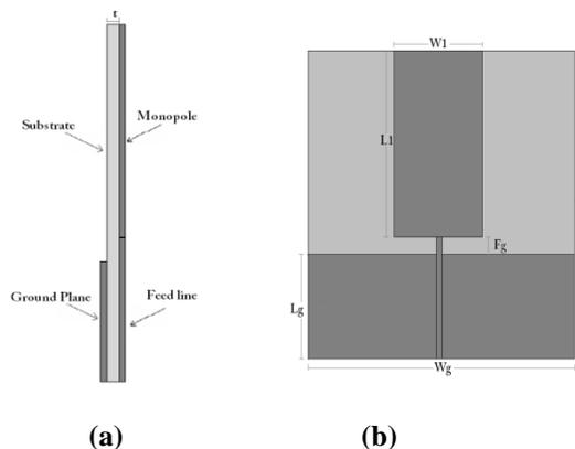
Figure 2: Showing the layout of a monopole antenna (a) Side view (b) Front view of antenna for frequency range from 3.34 to 12.1 GHz (bandwidth of 8.76GHz).
