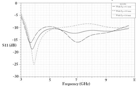
Figure 6. Showing the result of simulated return loss of rectangular antenna for different values of Fg
