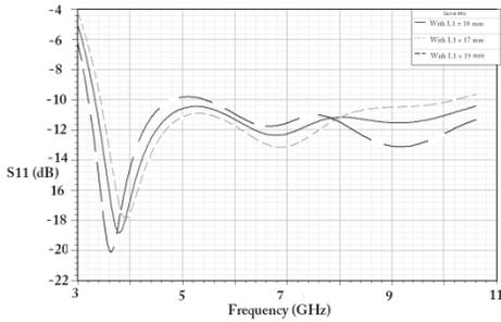
Figure 5. Showing the result of simulated return loss of rectangular antenna for different values of L1
