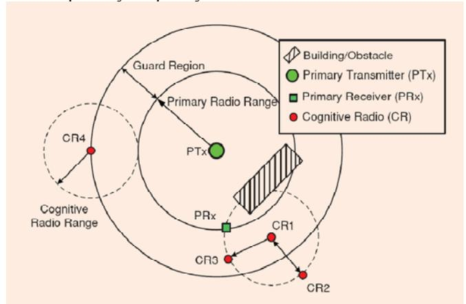
Fig. 4 The hidden terminal problem in CR networks, in which the guard region and the area covered by the primary radio range together form the protection region of the primary transmitter [4].
