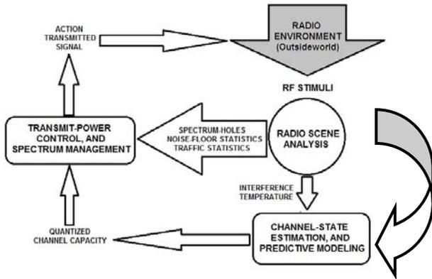
Fig. 2: Basic cognitive cycle which demonstrate three fundamental cognitive tasks.
