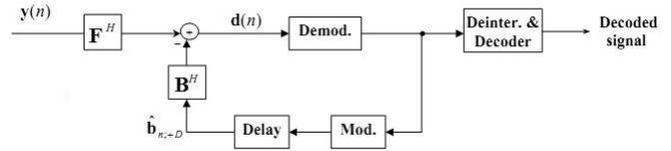
Fig. 3. Constrained MMSE-DFE
