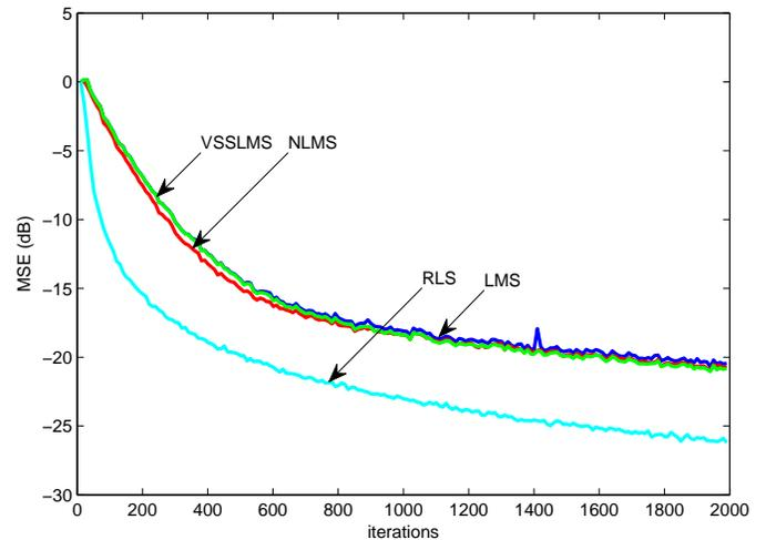
Fig. 7. MSE performance of various adaptive algorithms for a  $2 \times 2$  MIMO-DFE receiver.
