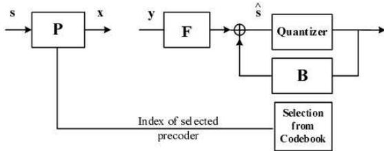
Fig. 5. Limited feedback MIMO ZF-DFE
