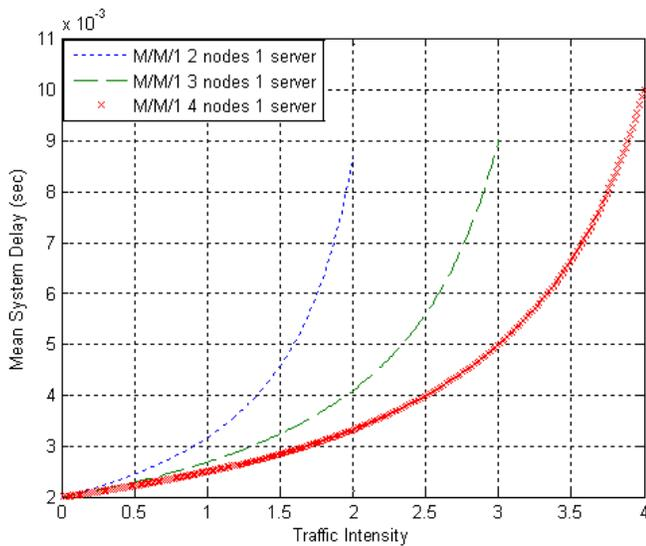
Figure 3: Mean System Delay for Scenario-I
