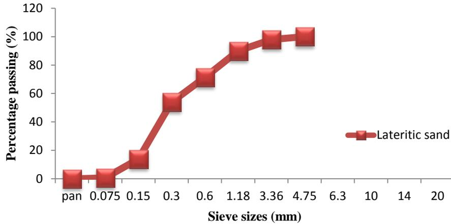
**Figure 2: Particle size distribution of fine aggregate (Lateritic sand)**
