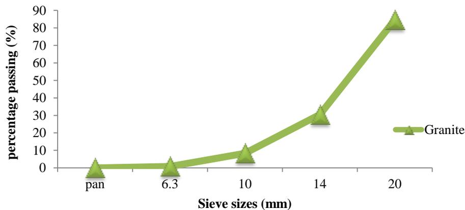
**Figure 3: Particle size distribution of coarse aggregate (granite)**
