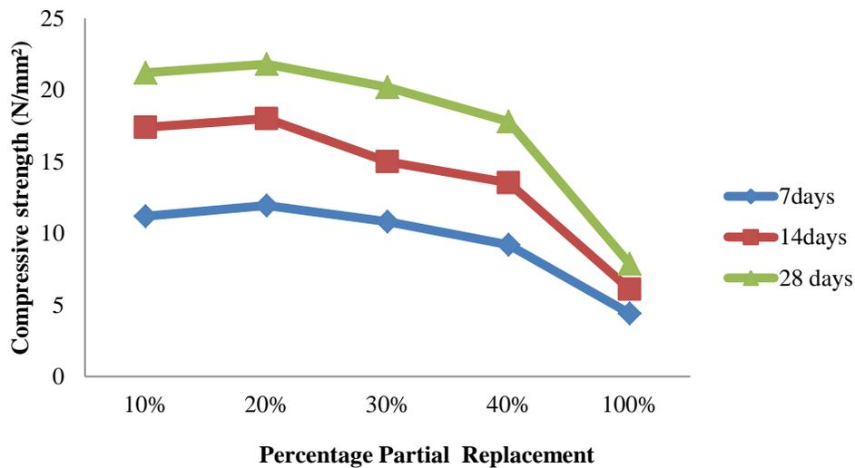
**Figure7:** Variation of compressive strength for 1:2:4 mix at various curing age with varying percentage replacement of fine and coarse aggregates with lateritic sand and periwinkle shell.
