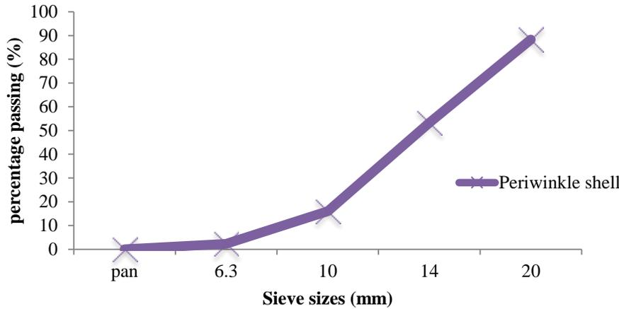
**Figure 4: Particle size distribution of coarse aggregate (Periwinkle shell)**
