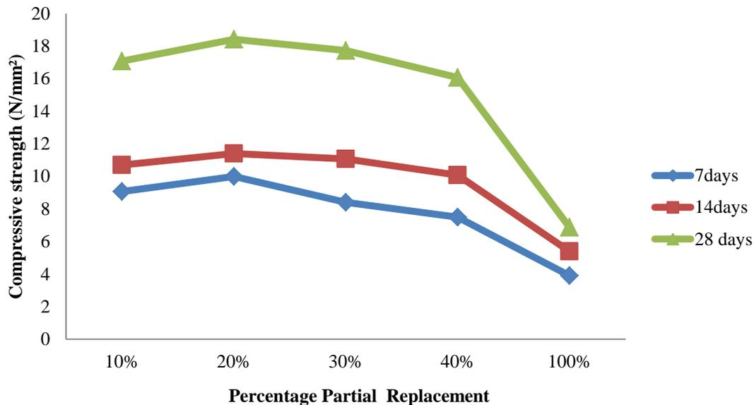
**Figure8:** Variation of compressive strength for 1:3:7 mix at various curing ages with varying percentage replacement of fine and coarse aggregates with lateritic sand and periwinkle shell.
