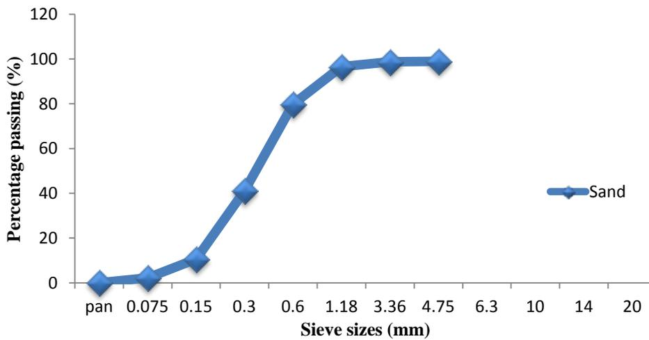
Figure 1: Particle size distribution of fine aggregates (sand)
