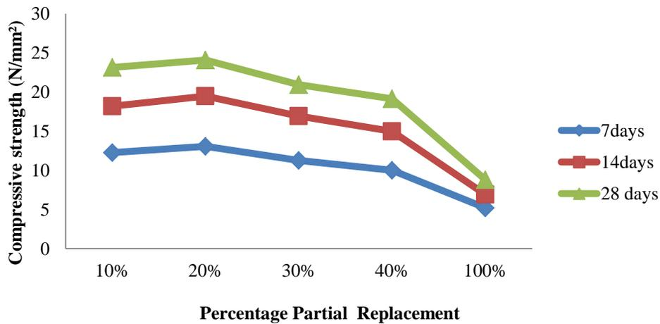
**Figure 6:** Variation of compressive strength for 1:1<sup>1</sup>/<sub>2</sub>:3 mix at various curing ages with varying percentage replacement of fine and coarse aggregates with lateritic sand and periwinkle shell.
