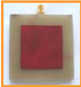
Figure 4. Front side of Fabricated Antenna
