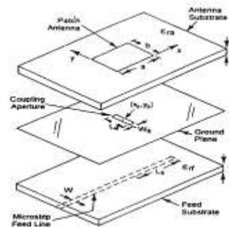
Figure 1. Exploded view of aperture coupled patch antenna
