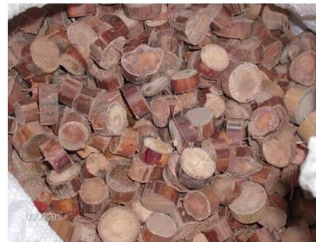
**Fig 1:** Sliced Rattan used in Concrete
