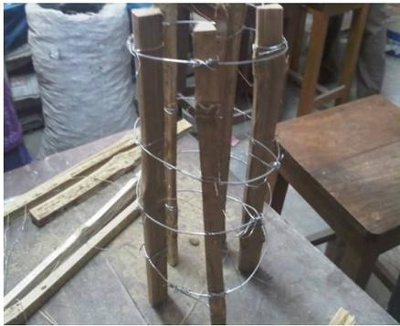
Fig 4: Bamboo encasement
