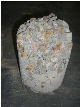
Fig 13: Crushed CR
