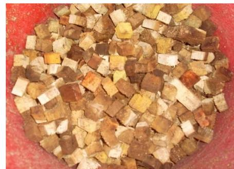
**Fig 2:** Sliced Wood used in Concrete
