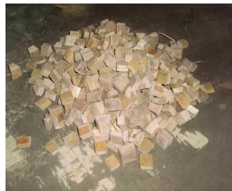
**Fig 3:** Sliced Bamboo used in Concrete
